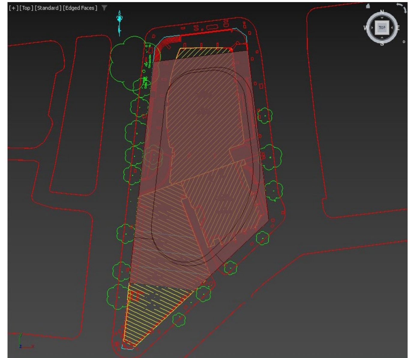
Image showing survey drawing from Project Surveyors at MGA 56 GDA2020 and 3D model of the proposed aligned to site boundary
